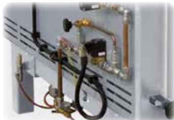
Gas lines and thermocouple at the chamber kiln
