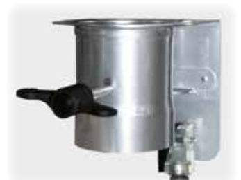
Semi-automatic air inlet flap for residual drying in chamber kilns up to 300 liters. The flap closes automatically at a set temperature and does not have to be closed manually after the drying phase.
