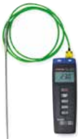
Temperature gauge for RAKU kiln 100, easy to operate, NiCr-Ni temperature sensor, display range 20 °C - 1200 °C, optional connection of second sensor with display changeover
