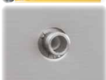
Observation hole in the kiln door (diameter 20 mm)
